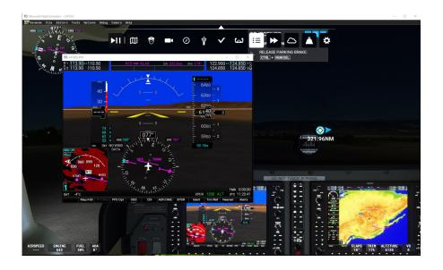
Drag the pop out panel to the G1000 simulator screen. After moving the pop out to the simulator screen, by holding the ALT + ENTER keys will toggle the pop out to full screen mode and dock the pop out panel to the simulator screen. Adjust the pop out window to fit the simulator screen by toggling full screen mode and re-adjusting the pop out window size.
